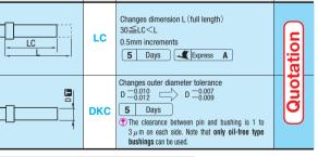
🕐 Use an oil-free type bushing for the pins modified by DKC alteration. Oil type bushings may cause scuffing because oil film is hard to form on them.
