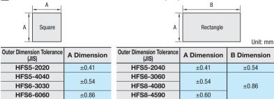
\*MISUMI Aluminum Extrusions are within JIS dimension tolerance above.
